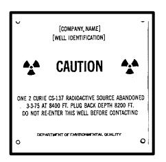
The size of the plaque should be convenient for use on active or inactive wells, e.g., a 7-inch square. Letter size of the word "CAUTION" should be approximately twice the letter size of the rest of the information, e.g., 1/2-inch and 1/4-inch letter size, respectively.
