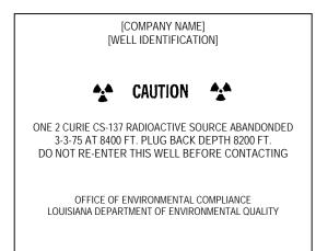
The size of the plaque should be convenient for use on active or inactive wells, e.g., a 7-inch square that is 3 mm (1/8-inch) thick. Letter size of the word "CAUTION" should be approximately twice the letter size of the rest of the information, e.g., 1/2-inch and 1/4-inch letter sizes, respectively.
